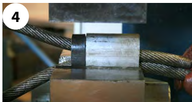
Mount in lubricated dies. T-LOC must be positioned next to T ferrule.
