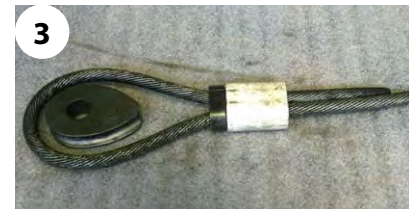
Incorporate thimble, if used. Further adjustment while swaging.
