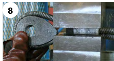
Swage T-LOC and ferrule (or first part of the ferrule, if the assembly is too long for the dies). Close dies.
