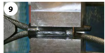
If a second swaging is required, open dies and swage the second part of the ferrule. Close dies.
