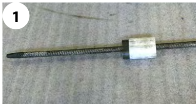
Thread ferrule and T-LOC on wire rope.
