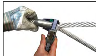
Always check the diameter after swaging.
