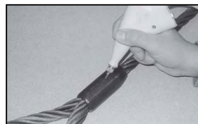
Marking of swaged sleeves should always be carried out according to ruling standards.
