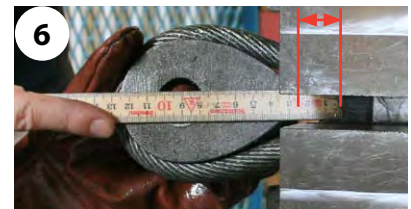
Measure. Distance T-LOC and solid thimble before swaging must be at least 2 times the nominal diameter. For pointed thimbles the distance can be reduced.
