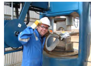
A refurbished 2000-ton swager, now equipped with rigging device
