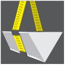
Protect any sharp edges on the load to avoid damaging
