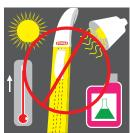
Store slings in a dry, clean and well ventilated area. Do not store: on the floor, in direct sun light, under UV light, near heat sources or chemical products etc.
