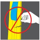
Defective slings must be destroyed immediately.
