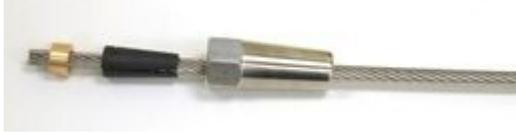
Place the brass pressure ring on the end of the cable. Make sure that the distance from the pressure ring to the end of the cable is 5mm.
