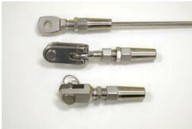
TECNI has a complete range of self-assembly, A4-AISI 316 marine grade stainless steel, swageless terminals - eyes, jaws, studs and toggles - all suitable for use with 1x19, 7x7 and 7x19 stainless steel wire rope.
