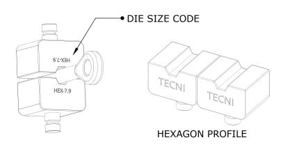
FOR SWAGING STAINLESS STEEL SWAGE FITTINGS (SEE PRE-SWAGE SIZE & AFTER SWAGE SIZE IN TABLE FOR SIZES BEFORE & AFTER SWAGING)
